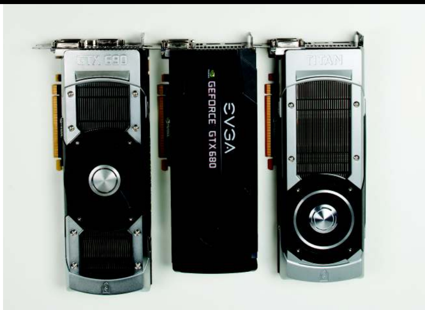
When it comes to length, the 10.5-inch Titan (right) lies in between the GTX 680 (middle) and the GTX 690 (left). It was designed to fit into rigs that can't accommodate the massive GTX 690.
